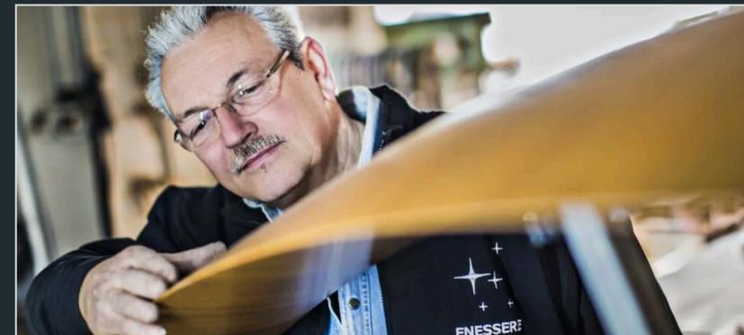
Paulownia wood comes from the Paulownia Tomentosa tree, known for its ecological characteristics: this tree grows in record time and produces 4 times more oxygen than other trees. Each wing of the Hercules wind turbine, is covered with 4000 handmade strips of Paulownia wood.
